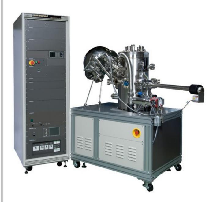
Monochromatic, micro-focused, scanning x-ray source provides excellent large area and superior micro-area spectroscopy performance.
