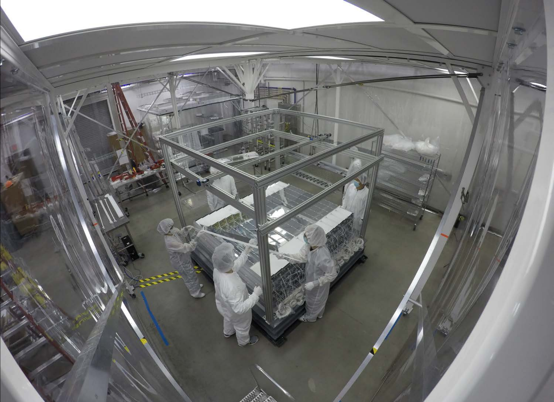
PROSPECT team assembling their antineutrino detector in one of Wright Laboratory's moveable clean rooms. – Frank Lopez
