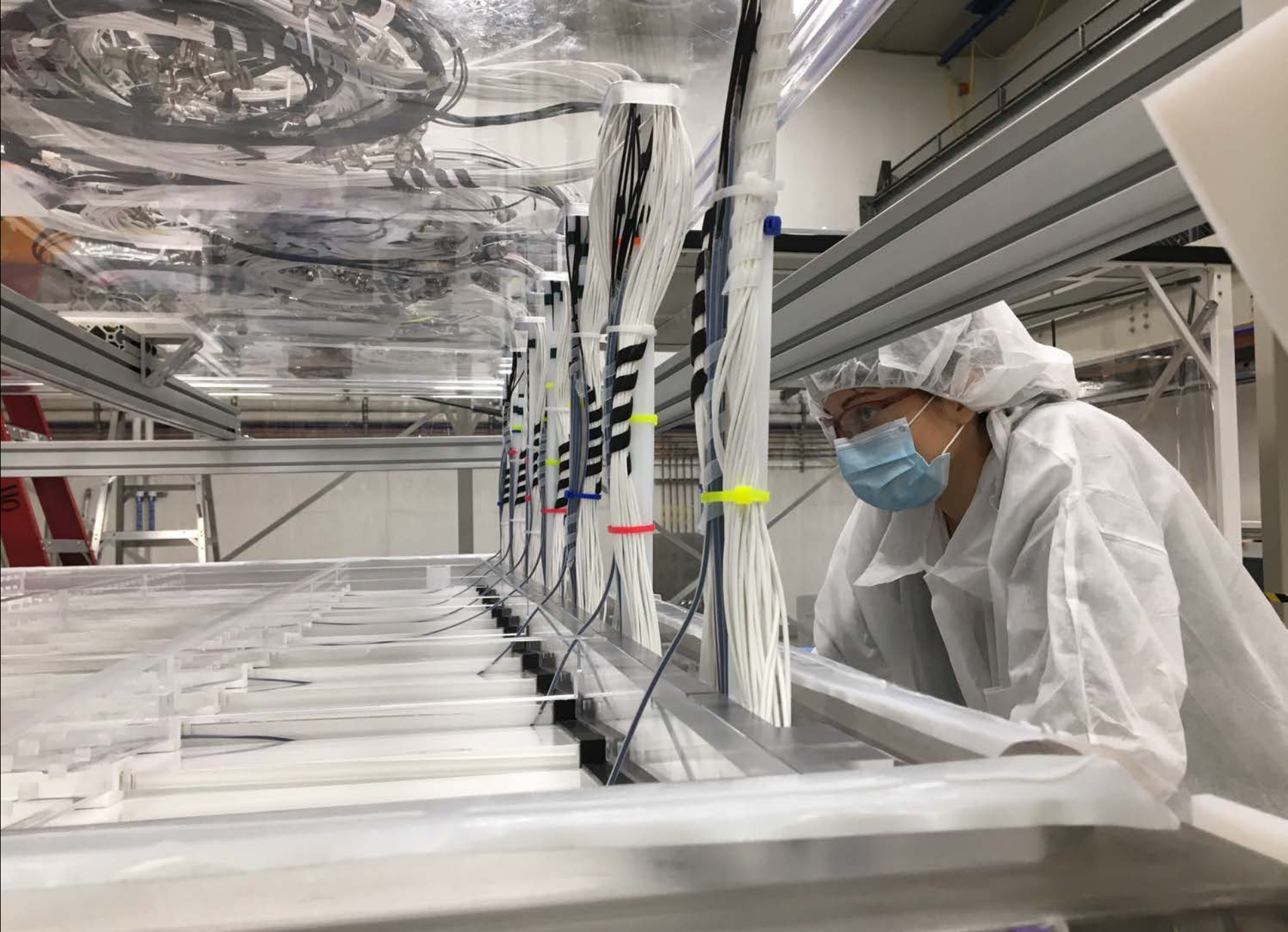
PROSPECT researcher, Danielle Norcini, carefully monitors the placement of the acrylic lid on their antineutrino detector. – Frank Lopez
