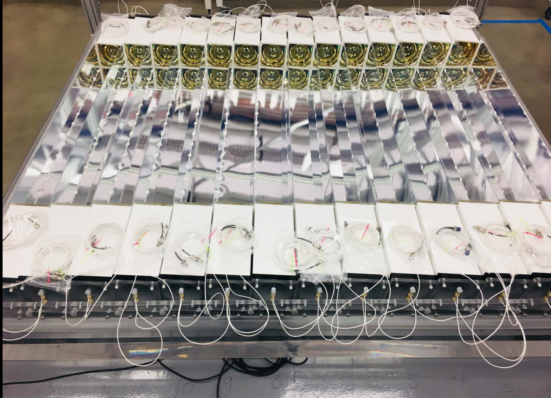
Bird's-eye view of the first layer of the PROSPECT neutrino detector built at the Yale Wright Laboratory. – Danielle Norcini
