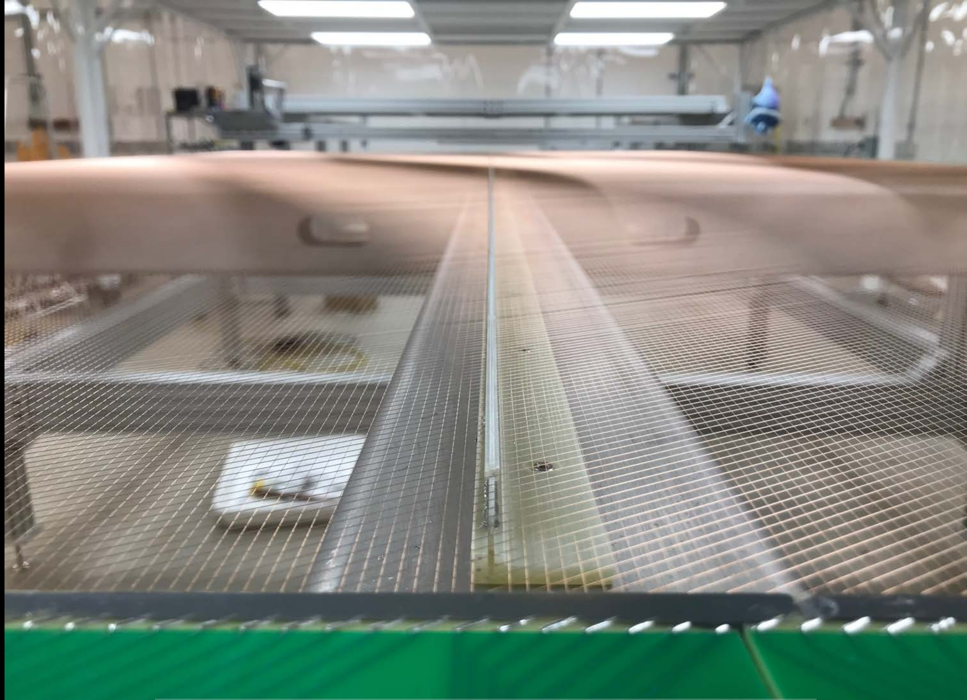
Detail of wire anode wire plane of the SBND's Time Projection Chamber. - SBND Collaboration
