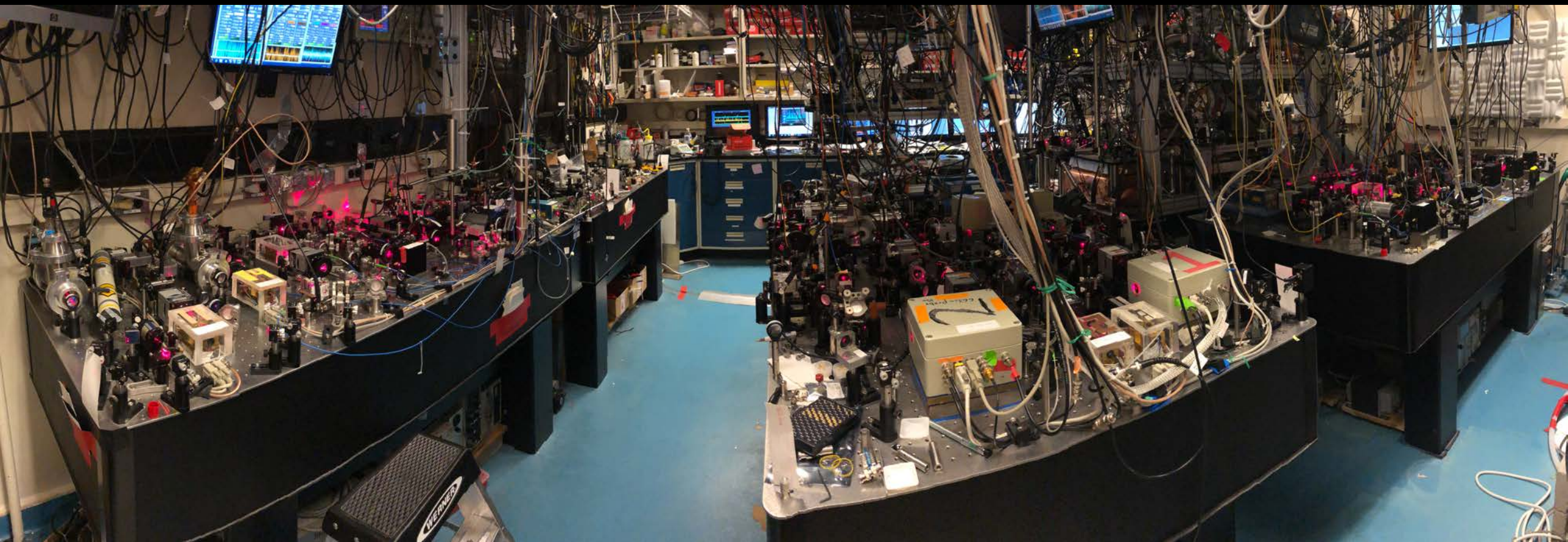
Apparatus for laser cooling and trapping of molecules. Twelve tunable lasers are frequency stabilized to \sim 1 part per billion and used to slow, cool, trap, and image molecules at temperatures as low as 50 millionths of a degree above absolute zero, inside a vacuum chamber maintained at less than one trillionth of atmospheric pressure. Six additional injection-seeded lasers and four tapered amplifiers provide the high laser power required, and a multitude of optical elements and cables provide the precise alignment and frequency control needed to successfully cool and trap molecules. - Matthew Steinecker
