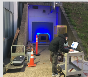
Jau Tung Chan ('21) measuring the distortion of the Fiberview Camera at 0°C outside Wlab. The calibration target is in the distance, illuminated by blue LED lights.
