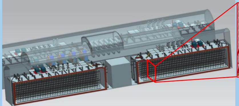
Dune LAr-TPC is segmented in units of suspend Anode/Cathode Plane Assemblies (APAs/CPAs) with 3.6 m maximum drift distance and a field of 0.5 kV/cm. Each APA reads out drifted ionization charge from a volume of liquid argon on either side of a sensor wire array. Data is recorded in the form of **high-resolution 2D-projected** views of charged particle trajectories in the liquid argon.
