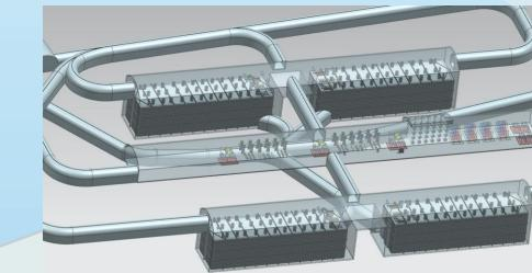
Dune far detector will consist in four 4 identical cryostats 62m (l) x 14m (w) x 15m (h) each instrumented with a **10kt fiducial volume** Liquid Argon TPCs. Each DUNE 10-kt LArTPC module is O(50x) scale-up w.r.t. largest LArTPC to date (ICARUS). The first 10kt module will begin data taking in 2026
