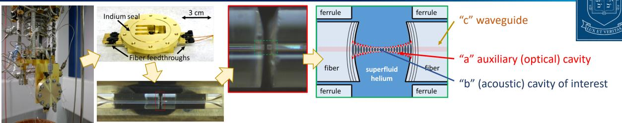
Detection of "c" photons w/ photodiode (quantity of interest: is there a phonon in the LHe?):
