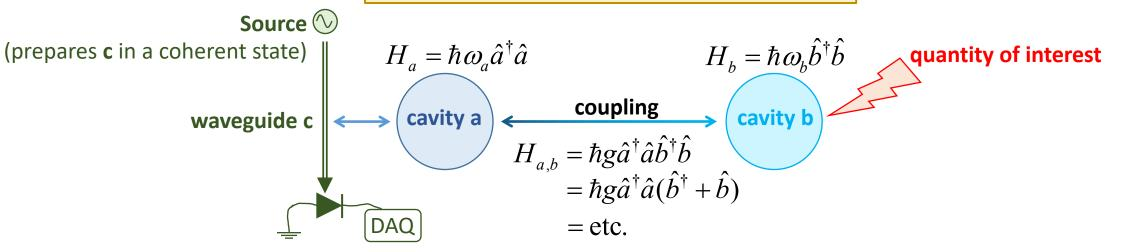
detects quanta of "c": single quanta resolution (PMT) or time-averaged flux of quanta (photodiode)
