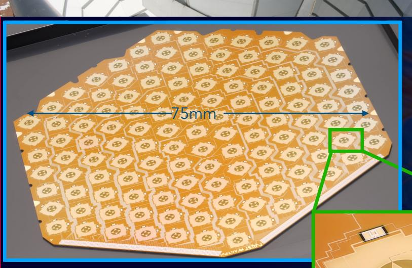
ACTPol wafer cooled to 100mK in a Dilution Refrigerator. Current receiver has 3000 pixels (6000 sensors) on three 6" wafers
