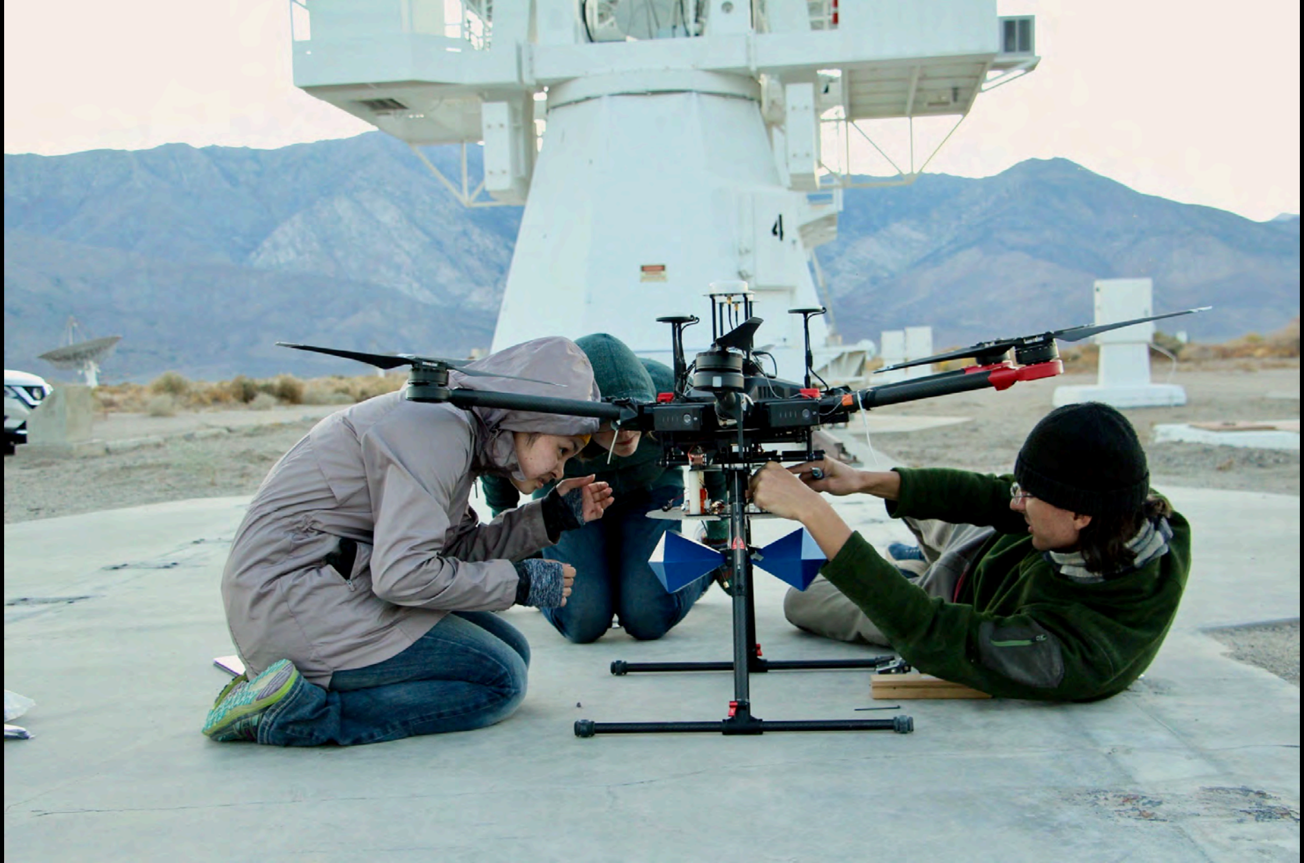
Prof. Laura Newburgh, Dr. Benjamin Saliwanchik, and Maile Harris (Pierson '22) tune scientific payload of Newburgh Lab Drone, before calibration flights at Owens Valley Radio Observatory.— Emily Kuhn
