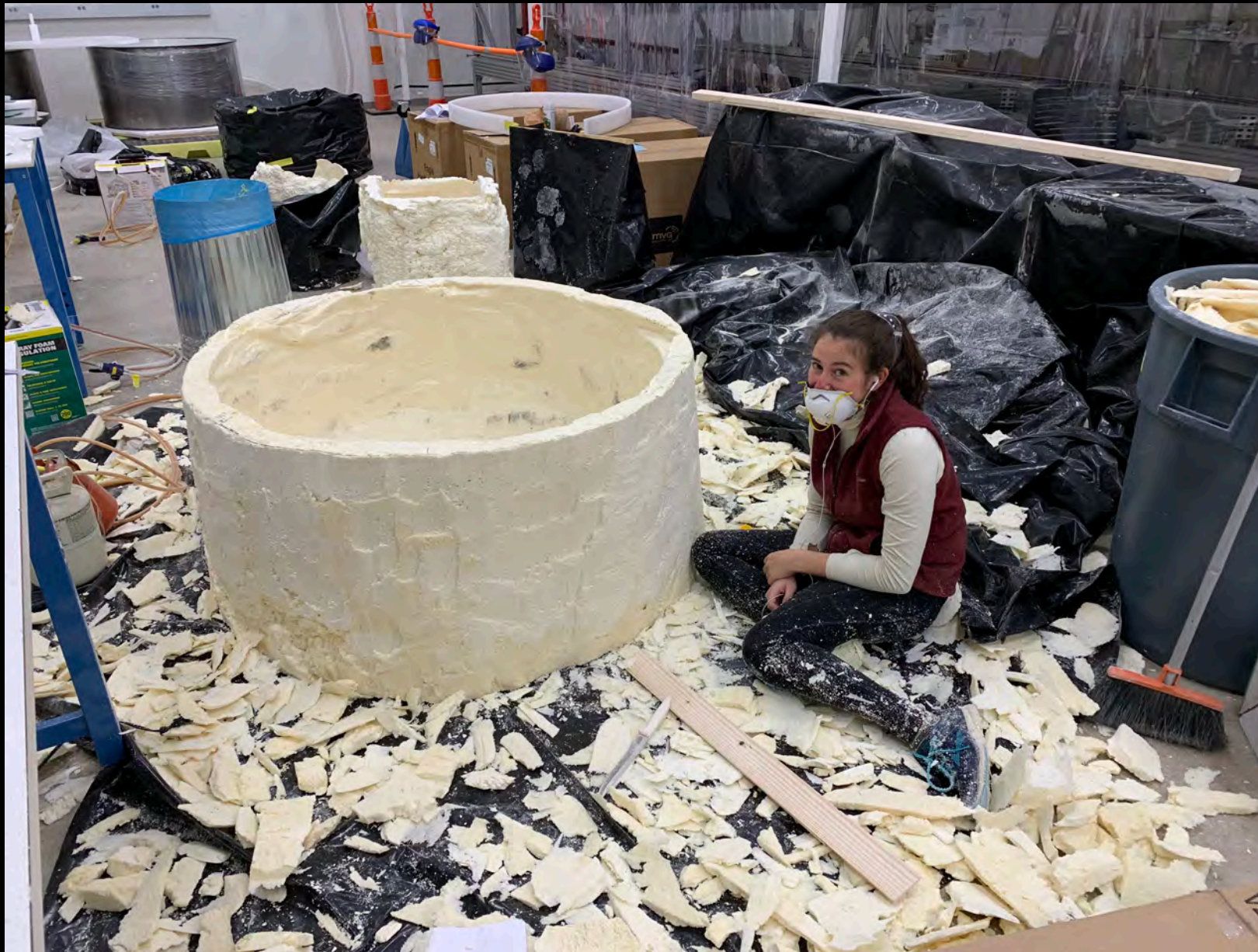
Self portrait: Emily, covered in shavings of polyurethane spray foam, after meticulously sculpting a container intended to hold 500L of liquid nitrogen for noise temperature testing. – Emily Kuhn
